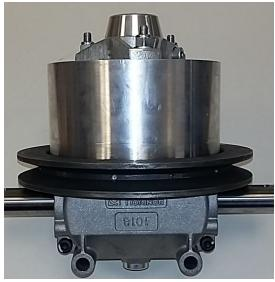
5. Once your pulley is at the desired height tighten the mount hub pinch bolt, followed by the hub mount bolts (you may wish to use thread lock). Care should be taken to make sure the pulley is not touching the axle or the top hat is not resting on the top of the T-drive.
