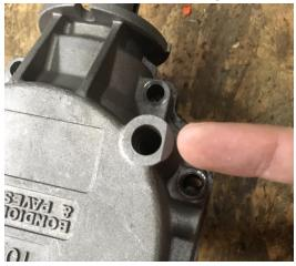
3. It may also be necessary to replace two bolts and nuts that bolt the T-drive together to gain extra clearance. Replacement lower profile button head bolts and slim nuts should be included on your T-drive kit, remove the original T-drive bolts and replace as in the pictures below.
